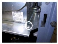
*Figure 4. Secure mechanism chassis to tray using two screws.*
