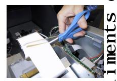
Figure 6-1. Cut paper between the roll and the printer feed path with scissors.
