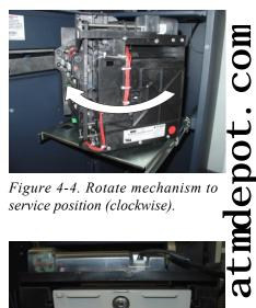
Figure 4-4. Rotate mechanism to service position (clockwise).
