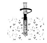
Figure 6. Drive anchor rod into capsule using hammer drill.
