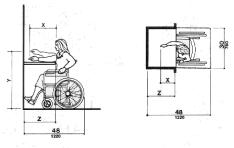
NOTE: x shall be ≼ 25 in (635 mm); z shall be ≥ x. When x < 20 in (510 mm), then y shall be 48 in (1220 mm) maximum. When x is 20 to 25 in (510 to 635 mm), then y shall be 44 in (1120 mm) miximum.
