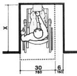
NOTE: If x > 24 in (610 mm), then an additional maneuvering clearance of 6 in (150 mm) shall be provided as shown.
