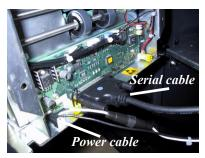
*Figure 3. Serial communication and DC power cables connected.*
