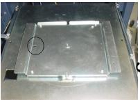
Figure 3. Turntable in cassette service position. Note that plate hole is to the left.
