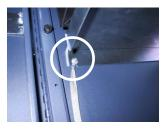
Grounding strap secured to dispenser tray mounting bolt.
