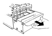
Figure 4-17. Removing note tray from the dispensing mechanism.
