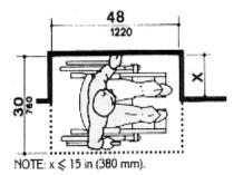
For a side approach, where the depth of the alcove is equal to or less than 15 inches (380 mm), the required clear floor space is 30 inches by 48 inches (760 mm by 1220 mm).
