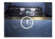
Figure 4-3. Pull release pin for swivel platform.
