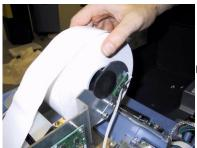
Figure 6-5. Place paper roll on bracket. Paper feeds from top of roll!
