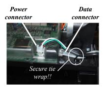
Figure 11. Data / power connections.
