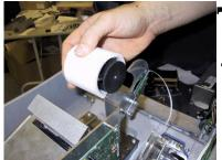
Figure 6-3. Removing paper roll from bracket.
