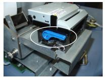
*Figure 6-10. Blue tension lever (correct position).*
