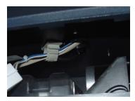
*Figure 12. Cables routed through cable clip.*
