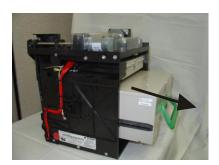
Figure 4-6a. Removing note cassette. (TDM-100)
