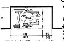
NOTE: If x > 15 in (380 mm), then an additional maneuvering clearance of 12 in (305 mm) shall be provided as shown.
